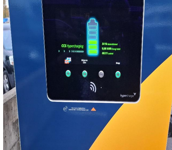
Figure 3: 150KW CCS Charger
